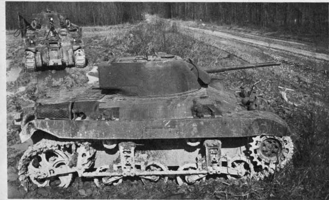
U. S. airborne tank the T-9E1, has a suspension very much like that of the M-5A1 (above). An added feature is the horizontal brace which supports the lightweight bogies. Fenders often alter the appearance of a tank's undercarriage. Here they cover the top of the track and partly hide two return rollers.
